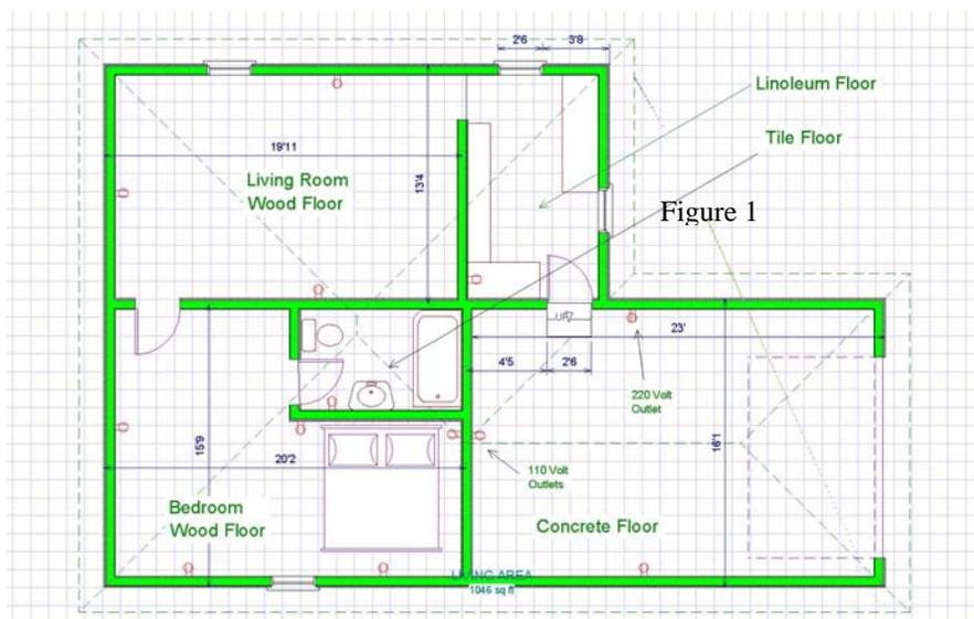
After the coating samples have passed inspection, proceed with the room farthest from the front door, the bedroom in this example. If furniture is in the rooms move to one side and coat and cure these areas first. Move the furniture onto the cured area remembering not
